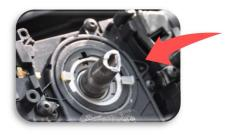
Steering column hollow and breakable with tools
